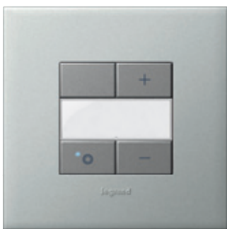
Dimmer actuator to control a load. There are two versions: • 300W multiload for connection "without neutral conductor"; • for ballast 0-10V with power max. 1000 W.
