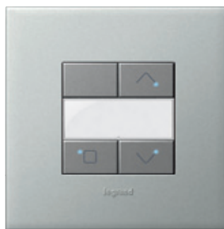
Dimmer actuator to control a load. There are two versions: • 300W multiload for connection "without neutral conductor"; • for ballast 0-10V with power max. 1000 W.
